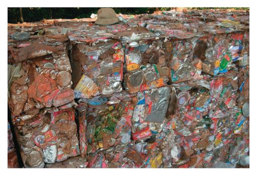
THESE CANS ARE MADE FROM STEEL COATED WITH A THIN LAYER OF TIN. BECAUSE TIN IS RELATIVELY UNREACTIVE, THE CANS WILL CORRODE MORE SLOWLY THAN CANS MADE OUT OF STEEL ALONE.
